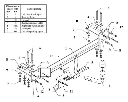
This towing hitch is designed to assembly in following cars: CHEVROLET LACETTI 4 doors, produced since 2005, catalogue no. X19 and is prepared to tow trailers max total weight 1200 kg and max vertical load 75 kg.
